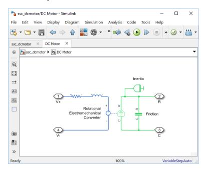
The following code implements the same model by means of a composite component, called DC Motor. The composite component uses the components from the Simscape Foundation library as building blocks, and connects them as shown in the preceding block diagram.
