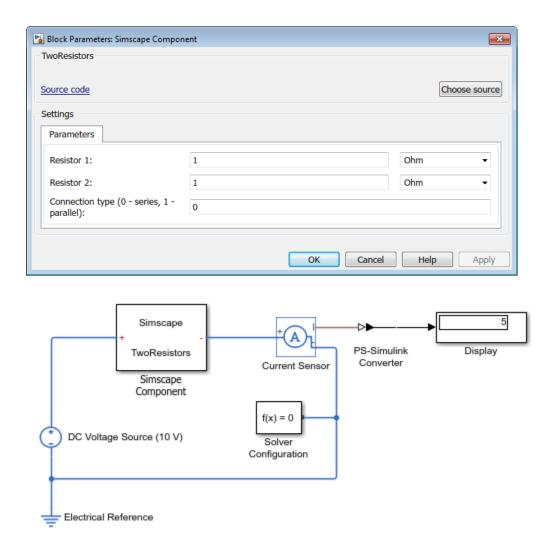
If you change the value of the **Connection type (0 - series, 1 - parallel)** parameter to 1, the resistors are connected in parallel, and the current is 20A.
